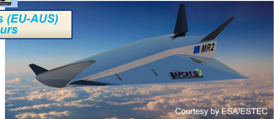
LAPCAT MR2.4 vehicle for passenger transportation (300 PAX, cruise at Mach 8, 32÷33 km altitude)
