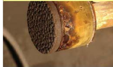
Without particles: Fissured surface pattern, samples slightly increased in thickness
