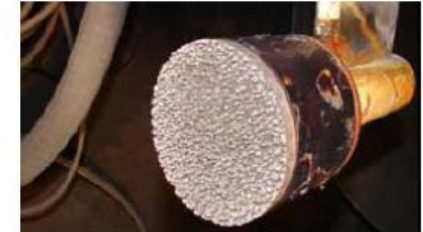
With 3 μm BN particles: Rough surface pattern, samples clearly reduced in thickness
