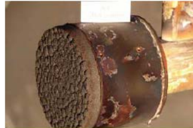
Without particles: Fissured surface pattern, samples slightly increased in thickness
