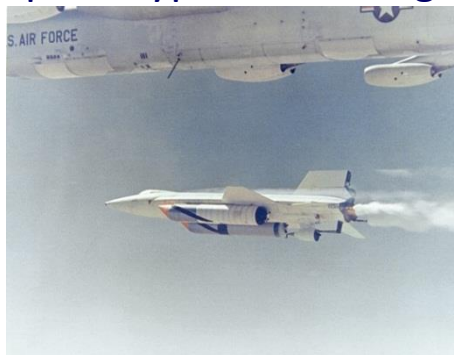
NASA Dryden Flight Research Center Photo Collection http://www.dfrc.nasa.gov/gallery/photo/index.html NASA Photo: EC08-1889 Date: 1967 Photo by: NASA photo X-15A-2 launch from B-52 with ablative coating and external tanks
