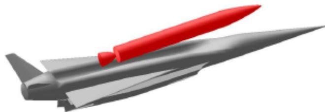
Stage 2 - Hydrogen fuelled scramjet accelerator
