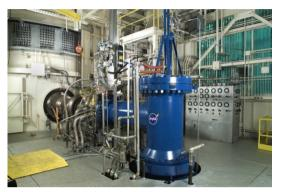
View of flow path for heated GN2 from the storage heater below deck, through the oxygen injection and GN2 diluent sections, providing precise mixture ratios and temperature control, to the expansion nozzle and altitude chamber (background).
